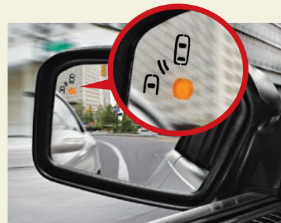
LANE ALERT A warning light on this Lincoln MKZ Hybrid shows when a car is in your blind spot, so you don't try to change lanes.
