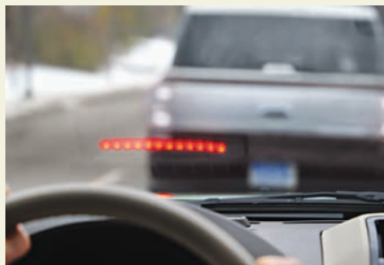
SEEING THE LIGHT The bright band of lights in Ford and Mercedes-Benz cars creates an effective warning signal.
